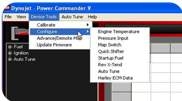
Engine temp - Displays engine temp either via the J1850 port or thru the 0-5v input
