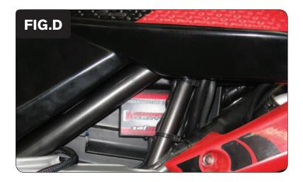
5 Install the PCV to the right side of the airbox. Use the supplied Velcro to secure the unit in place.
