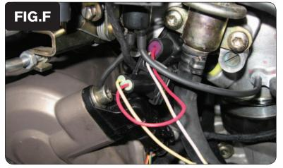
10 Plug the pair of PCV leads with ORANGE colored wires in-line of the stock wiring harness and the front fuel injector (Fig. F).
