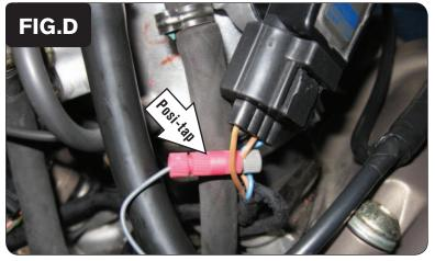
7 Use the supplied Posi-tap to attach the single GREY wire of the PCV to the stock BROWN/WHITE wire of the bike's Throttle Position Sensor wiring harness (Fig. D).
