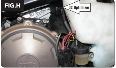
13 Plug the supplied O2 Optimizer in-line of the stock O2 sensor and stock wiring harness (Fig. H). With the supplied Velcro, secure the O2 Optimizer in place.
