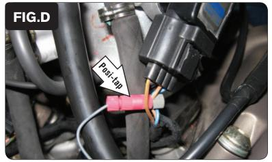
Use the supplied Posi-tap to attach the single GREY wire of the PCV to the stock BROWN/WHITE wire of the bike's Throttle Position Sensor wiring harness (Fig. D).
