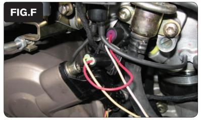
Plug the pair of PCV leads with ORANGE colored wires in-line of the stock wiring harness and the front fuel injector (Fig. F).
