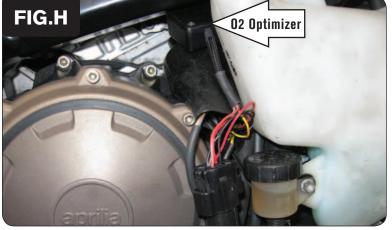
Plug the supplied O2 Optimizer in-line of the stock O2 sensor and stock wiring harness (Fig. H). With the supplied Velcro, secure the O2 Optimizer in place.
