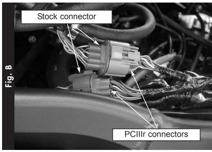
Plug the PCIII connectors in-line of the stock connector (Fig. B).
