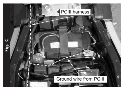
Attach the ground wire from the PCIII to the NEGATIVE side of the battery (Fig. C).
