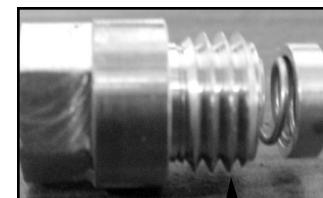
Install the stock needle retainer on top of the Dynojet needle, e-clip and washer.
