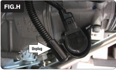
12 Unplug the stock O2 sensor from the main wiring harness on the left hand side (Fig. G).
