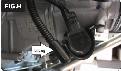
13 Unplug the stock O2 sensor from the main wiring harness on the right hand side (Fig. H).
