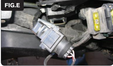
Plug the pair of 3-pin connectors from the PCV in-line of the bike's TPS and the stock wiring harness (Fig. E).
