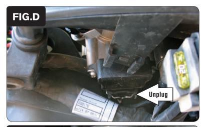
On the right side of the bike, unplug the stock wiring harness from the Throttle Position Sensor on the side of the throttle body (Fig. D).
