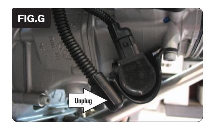
13 Unplug the stock O2 sensor from the main wiring harness on the right hand side (Fig. G).
