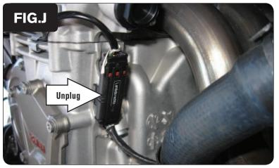
14 Unplug the stock O2 sensor on the right side of the engine (Fig. J).
