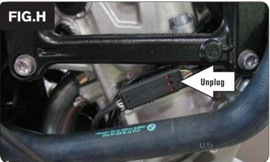
13 Unplug the stock O2 sensor on the left side of the engine (Fig. H).
