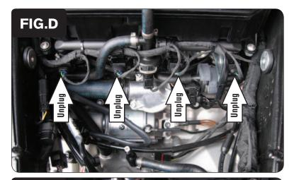
8 Unplug the stock wiring harness from each fuel injector (Fig. D).
