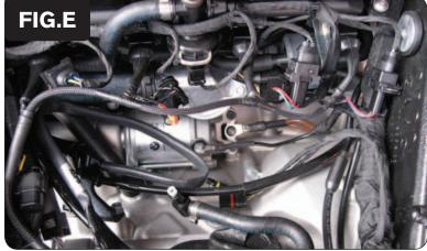
9 Plug the PCV harness in-line of the stock wiring harness and each fuel injector (Fig. E).
