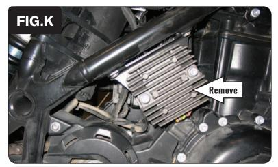
Remove the regulator/rectifier to access the O2 sensor connection behind it (Fig. K).
