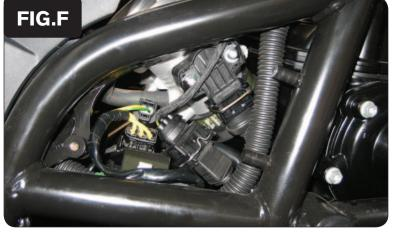
Plug the PCV wiring harness in-line of the stock wiring harness and both of the fuel injectors (Fig. D).
