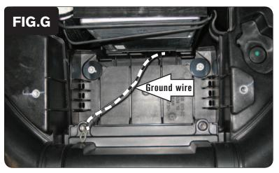
Reinstall the airbox while routing the ground wire of the PCV through the battery location (Fig. G).
