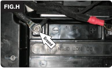
Reinstall the battery. Connect the ground wire from the PCV with the small ring lug to the negative (-) terminal of the bike's battery (Fig. H).
