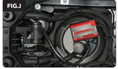
14 Secure the PCV in place using the supplied Velcro (Fig. J).
