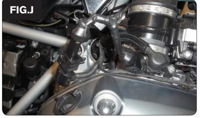
14 Plug the pair of PCV injector leads with the YELLOW colored wires in-line of the right fuel injector and the stock wiring harness (Fig. J).
