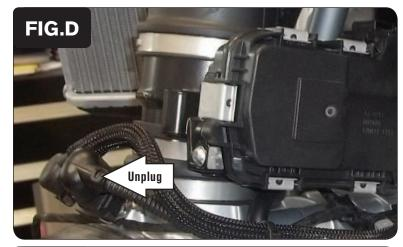
9 Unplug the stock wiring harness from the left fuel injector (Fig. D).
