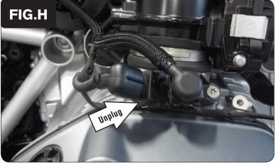
13 Unplug the stock wiring harness from the right fuel injector (Fig. H).
