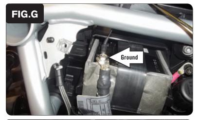
12 Secure the PCV ground wire with the ring lug to the negative (-) terminal of the bike's battery (Fig. G).
