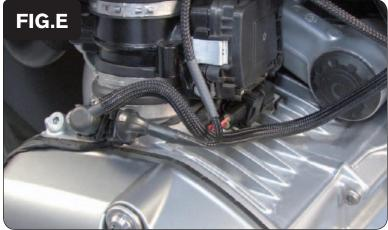
Plug the pair of PCV injector leads with the ORANGE colored wires in-line of the left fuel injector and the stock wiring harness (Fig. E).
