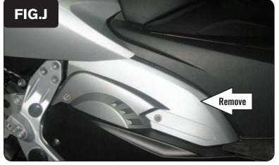
12 Remove the cover on the right side of the scooter (Fig. J).
