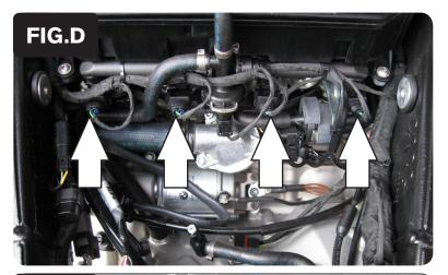
7 Unplug the stock wiring harness from each injector (Fig. D).
