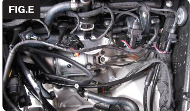
8 Plug the PCV harness in-line of the stock wiring harness and injectors (Fig.E).
