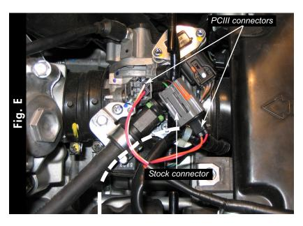
Plug the harness from the PCIII in-line of the injector and stock wiring harness (Fig. E).
