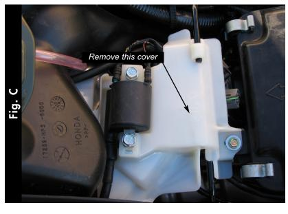
4 Remove the white cover over the throttle body (Fig. C).
