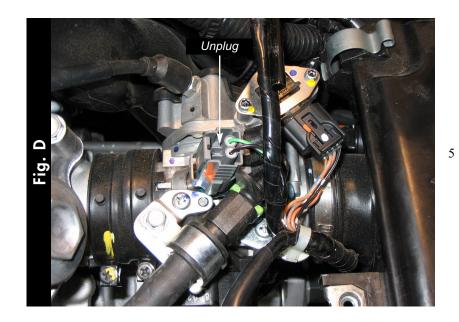
Unplug the stock wiring harness from the injector (Fig. D).
