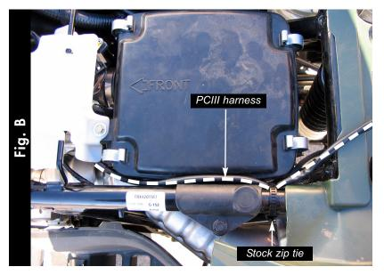
Route the PCIII harness along the left hand side of the quad (Fig. B).
