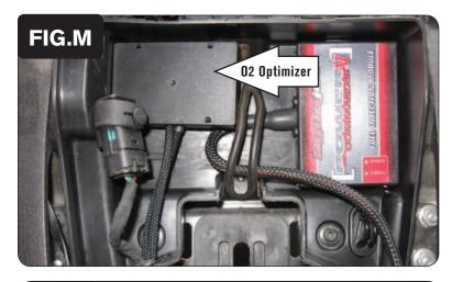
20 Using the supplied Velcro, secure both the PCV module and the O2 Optimizer module in the tail section.
