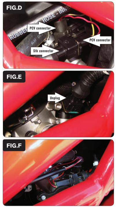
5 Plug the pair of PCV leads with YELLOW colored wires in-line of the rear fuel injector and the stock wiring harness (Fig. D).
