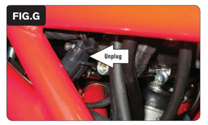
9 Locate and unplug the stock Throttle Position Sensor.
