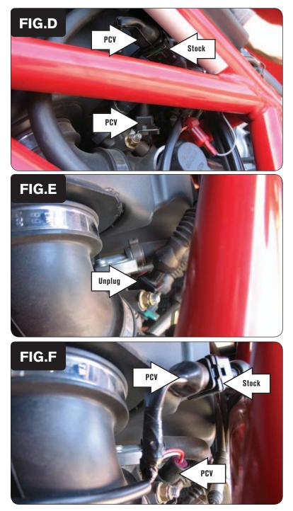
6 Plug the pair of PCV leads with YELLOW colored wires in-line of the rear fuel injector and the stock wiring harness (Fig. D).
