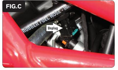
Unplug the stock wiring harness from the rear fuel injector (Fig. C).
