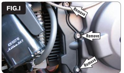
Remove the BLACK plastic engine cover on the left side of the bike by removing the 3 bolts (Fig. I).
