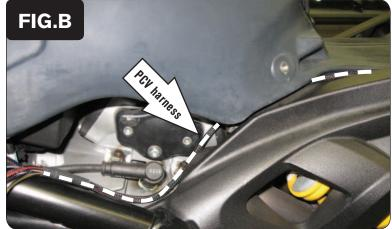
Continue routing the PCV harness along left hand side of the frame (Fig. B). 3
