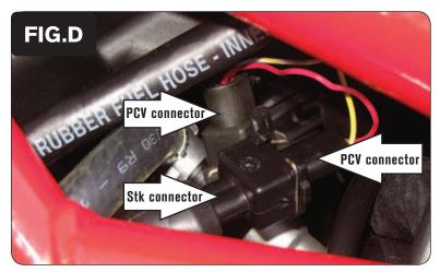
Plug the pair of PCV leads with YELLOW colored wires in-line of the rear fuel injector and the stock wiring harness (Fig. D).
