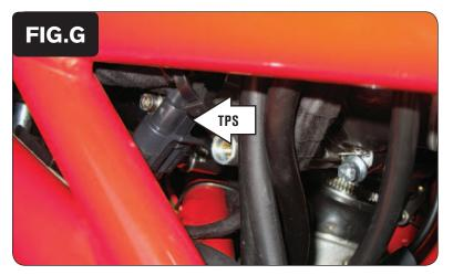
8 Locate and unplug the stock Throttle Position Sensor.
