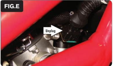
6 Unplug the stock wiring harness from the front fuel injector (Fig. E).
