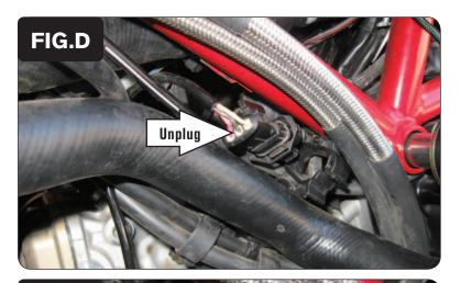
7 Locate the front ignition coil connection and unplug it (Fig. D).
