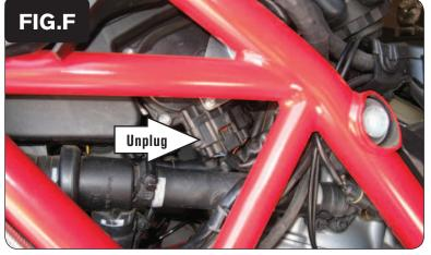
9 Unplug the stock wiring harness from the Throttle Position Sensor (Fig. F).
