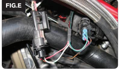
Plug the pair of PCV connectors with the GREEN colored wires in-line of the stock front ignition coil connectors (Fig. E).
