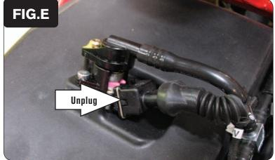
9 Unplug the stock wiring harness from the rear fuel injector (Fig. E).
