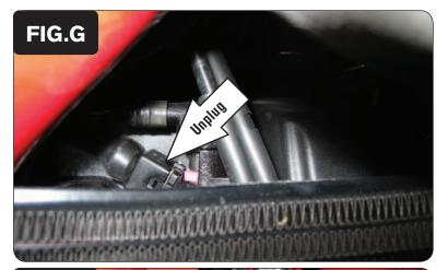
12 Unplug the stock wiring harness from the front fuel injector (Fig G).
