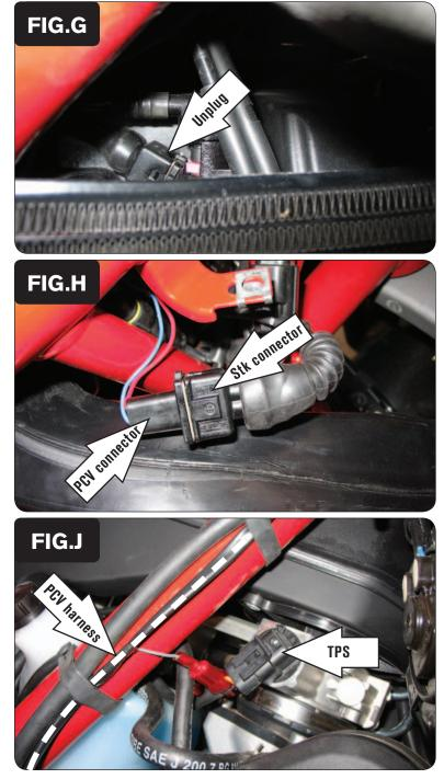
11 Unplug the stock wiring harness from the front fuel injector (Fig G).
