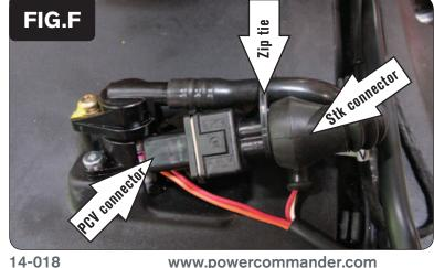
Route the PCV along the right hand side of the subframe. Secure the PCV harness to the subframe using the 2 large supplied zip-ties (Fig. D)
