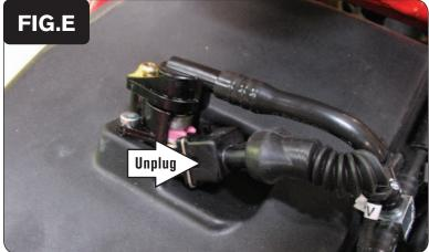
8 Unplug the stock wiring harness from the rear fuel injector (Fig. E).
