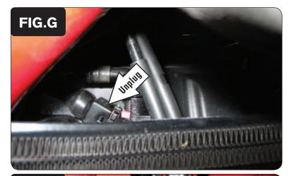
11 Unplug the stock wiring harness from the front fuel injector (Fig. G).
