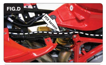
7. Route the PCV along the right hand side of the subframe. Secure the PCV wiring harness to the subframe using the 2 larger supplied zip ties (Fig. D).
