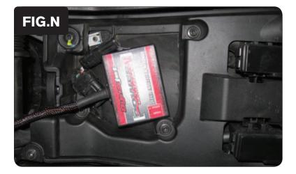
20 Secure the PCV in the area under the seat using the supplied Velcro (Fig. N).
