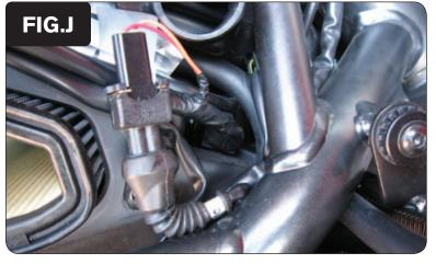
Plug the pair of PCV leads with ORANGE colored wires in-line of the stock wiring harness and the front fuel injector (Fig. J).
