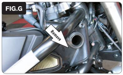
9 Remove the inner cover (Fig. G).
