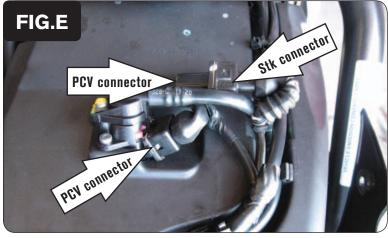
Plug the pair of PCV leads with YELLOW colored wires in-line of the rear fuel injector and the stock harness (Fig. E).
