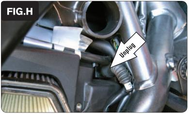
10 Unplug the stock wiring harness from the front fuel injector (Fig. H).
