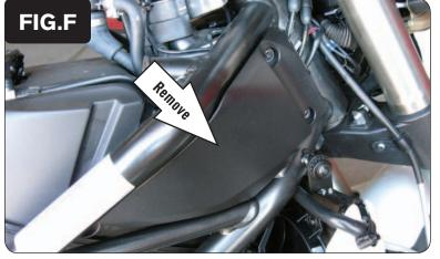
Remove the right hand side frame cover (Fig. F).
