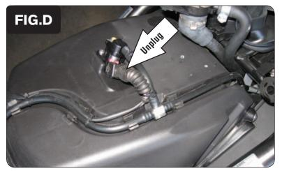
6 Unplug the stock wiring harness from the rear fuel injector (Fig. D).
