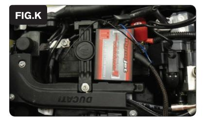
18 Use the supplied Velcro to secure the PCV module to the top of the battery (Fig. K).
