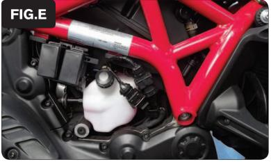
8 Plug the PCV in-line of the stock CPS and wiring harness.
