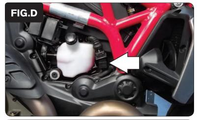
7 Unplug the stock Crank Position Sensor (Fig. D).
