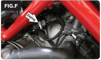
Beneath the rear of the fuel tank on the left side of the bike, locate and unplug the stock Fuel Injector connector and the stock Throttle Body Servo connector for the Vertical cylinder.
