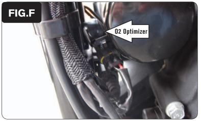
Locate the front stock O2 sensor connection. This is located in front of the oil filter. Unplug the O2 sensor from the wiring harness.
