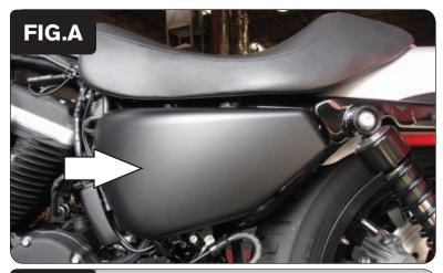
1 Remove the seat, left side cover and battery (Fig. A).
