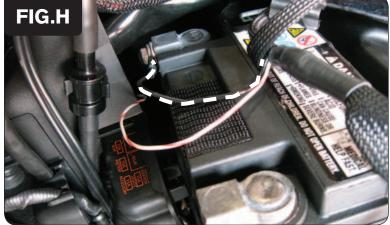
Reinstall battery. Attach the ground wire of the PCV to the negative side of the battery (Fig. H).
