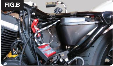
2 Route the large connectors of the PCV harness underneath the frame tube to the area under the seat (Fig. B).
