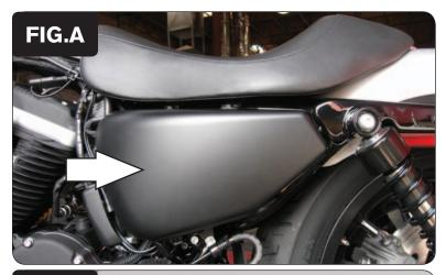
Remove the seat, left side cover and battery (Fig. A).
