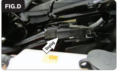
6 Locate and unplug the stock connector for the bike's rear cylinder O2 sensor (Fig. D).
