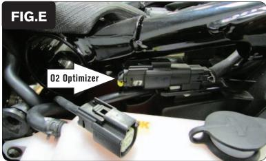
Plug the supplied BLACK O2 Optimizer into the bike's wiring harness in-place of the stock O2 sensor (Fig. E).
