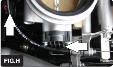
9 Unplug the stock wiring harness from the front injector and Throttle Position sensor (Fig. H).
