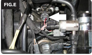
6 Unplug the stock wiring harness from the rear injector (Fig. E).
