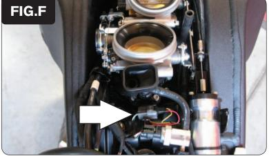
Plug the YELLOW colored wires from the PCV in-line of the stock wiring harness and rear injector (Fig. F).
