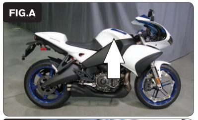
1 Remove both cosmetic covers around the air box (Fig. A).
