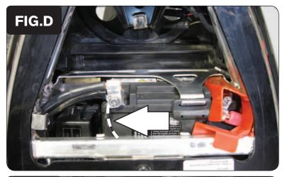
5 Attach the ground wire of the PCV to the negative side of the battery (Fig. D).
