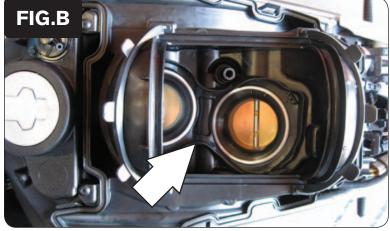
2 Remove the stock air box lid, air box base, and rubber seal around throttle bodies (Fig. B).
