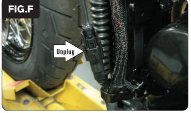
10 Locate and unplug the stock connector for the bikes front O2 sensor (Fig. F).
