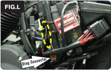
Plug the 12-volt power supply cable from the Auto-tune module into the bike's diagnostic connector (Fig. K).
