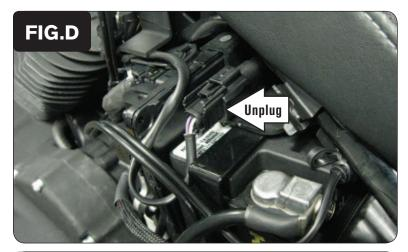
8 Locate and unplug the stock connector for the bikes rear O2 sensor (Fig. D).
