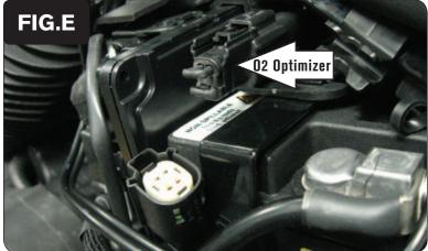
9 Plug one of the supplied O2 Optimizers into the stock wiring harness in place of the stock O2 sensor (Fig. E).
