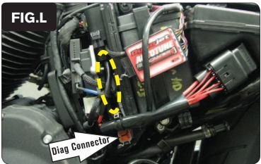
18 Plug the 12-volt power supply cable from the Auto-tune module into the bike's diagnostic connector (Fig. K).
