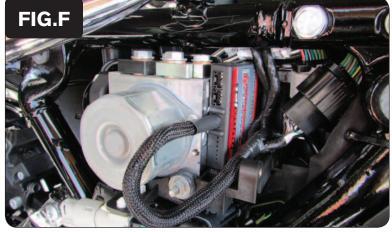
Secure the PCV under the right hand side cover using the supplied Velcro.
