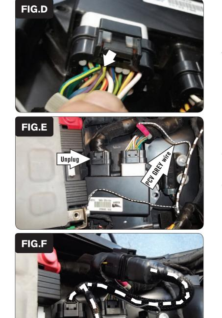
4 Locate the stock PURPLE/YELLOW wire on the ECU connector going to the GREY ECU connector input (Fig. D).
