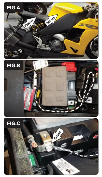
Remove the rider's seat and the covering above the airbox directly in front of the rider's seat (Fig. A).
