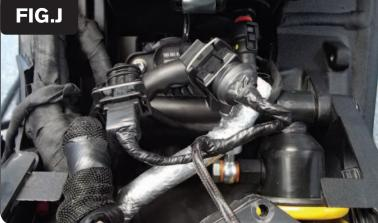
8 Route the pair of 3-pin connectors on the PCV wiring harness forward and behind the plastic panel directly rear of the airbox that holds the bank angle sensor (Fig. G).
