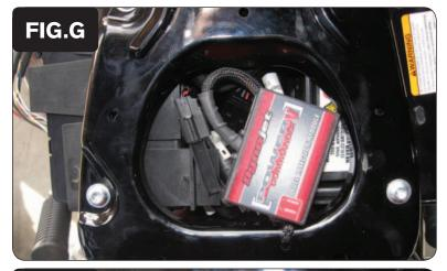
12 Install the PCV in the opening of the frame under the seat (Fig. G).
