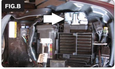
3 Unplug the stock wiring harness from the ECM (Fig. B).
