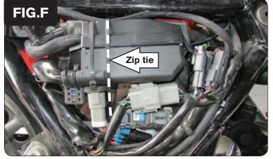
12 Use the supplied zip tie to secure the set of connectors to the ECU tray (Fig. F).
