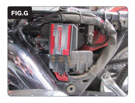
Use the supplied velcro to secure the PCV under the left hand side cover (Fig G).
