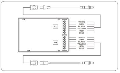
13 Plug the Dynojet O2 Optimizer (WHITE) into the stock wiring harness (Fig. G).
