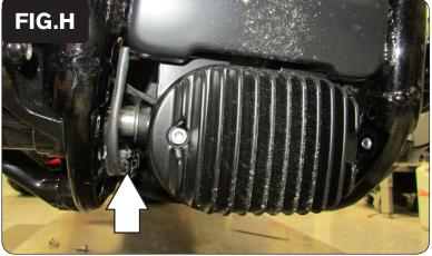
12 Locate the stock Rear O2 sensor connection and unplug it (Fig. G).
