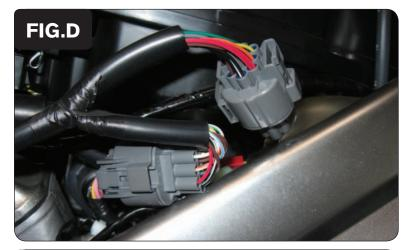
Plug the PCV wiring harness in-line of the stock wiring harness and injectors (Fig. D).
