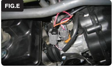
9 Plug the connectors from the PCV in-line of the stock injectors and wiring harness (Fig. E).
