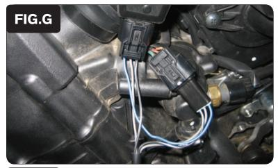
11 Plug the connectors from the PCV in-line of the TPS and stock wiring harness (Fig. G).
