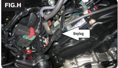
Locate the stock O2 sensor wiring harness connection to the main wiring harness (Fig. H).
