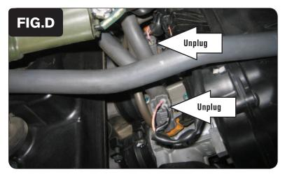
8 Unplug the stock wiring harness for cylinders #2 and #3 (Fig. D).
