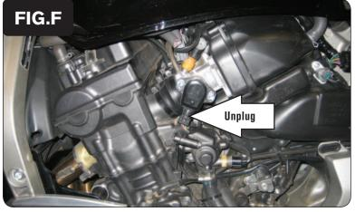
Locate the Throttle Position Sensor on the left hand side of the throttle bodies.
