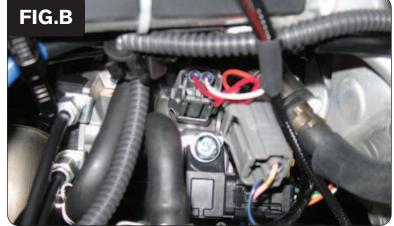
3 Connect the PCV in-line of the stock wiring harness and the injector (Fig. B).
