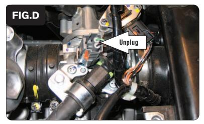
5 Unplug the stock wiring harness from the injector (Fig. D).
