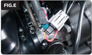
6 Plug the harness from the PCV in-line of the injector and stock wiring harness (Fig. E).
