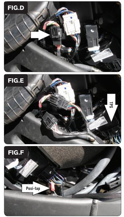
8 Locate the BLACK 12-pin connector on the left side of the airbox (Fig. D). Unplug this connector.
